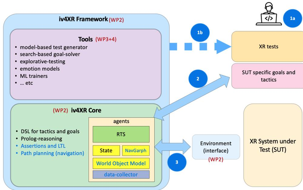
Fig.1: Top-level architecture of iv4XR framework
